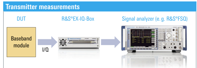
FIG 4 The analyzers' wide range of functions for analyzing digital baseband signals of all important standards is available, for example, for performing transmitter measurements on baseband modules.
