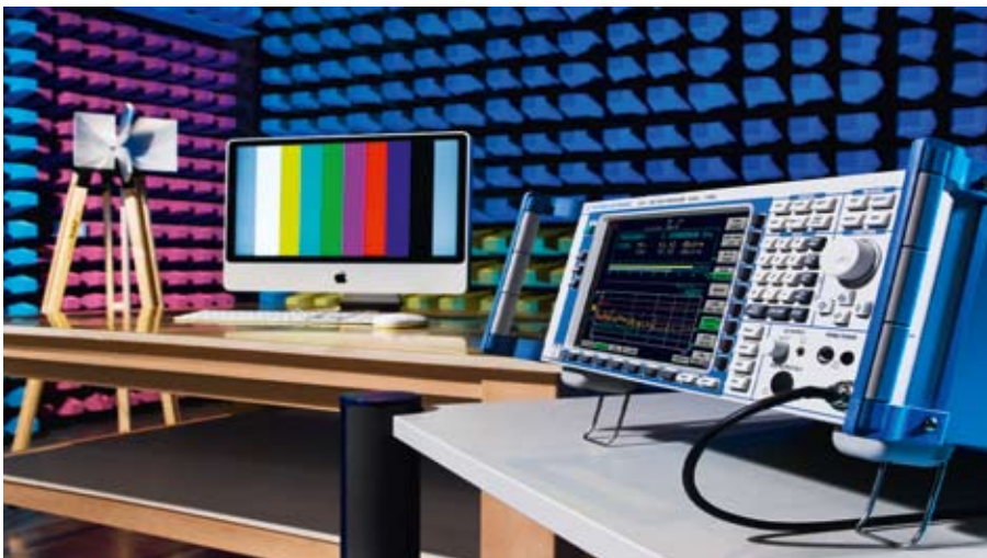
Measurement of radiated disturbances in line with the product standard CISPR 22:2005 Amend. 1:2005/ EN 55022:2006 Amend. 1:2007 for information technology equipment (ITE) in the range from 1 GHz to 6 GHz using the R&S®ESC17 EMI test receiver and the R&S®HF907 double-ridged waveguide horn antenna.
