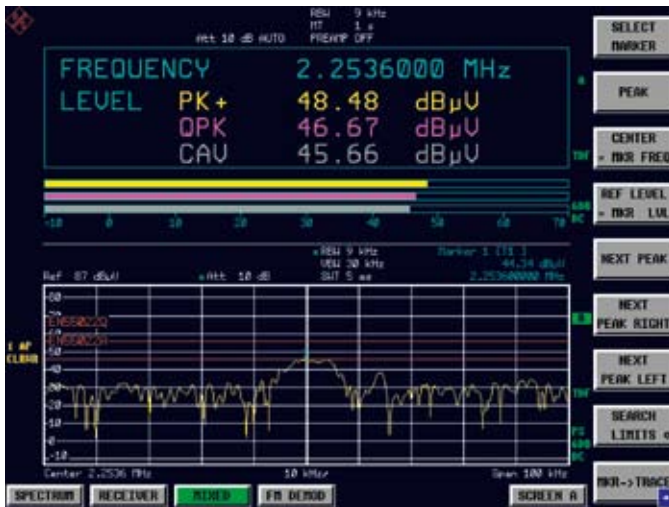
Mixed-mode display: bargraph measurement and spectrum. The standard-compliant measurement in the bargraph display and the fast sweep are shown simultaneously.
