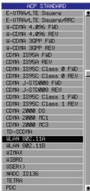
Overview of preprogrammed ACP standards for adjacent channel power ratio (ACPR) measurement, which is a power measurement specified in many mobile radio standards.
