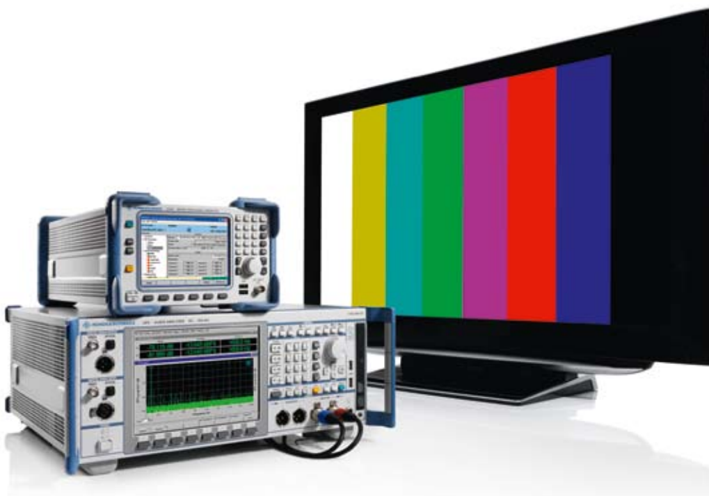
Audio test setup consisting of the R&S®DVSG, a TV set and the R&S®UPV.
