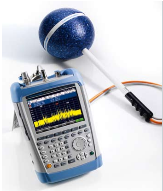
Field-strength measurements using the R&S®TS-EMF isotropic antenna.
