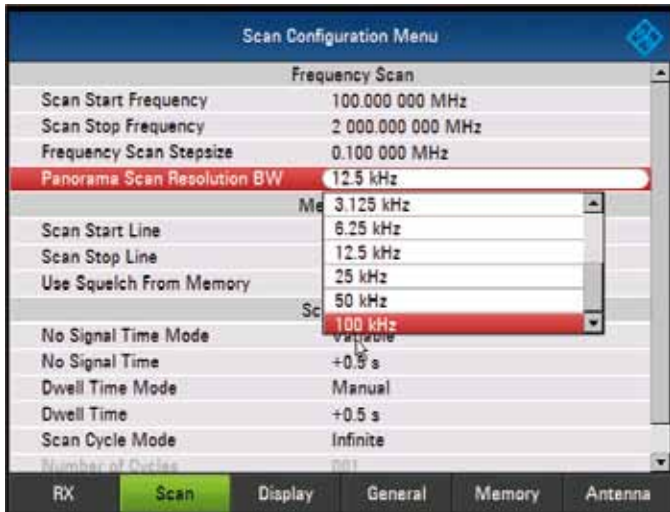
Structure of R&S®PR100 configuration menus.
