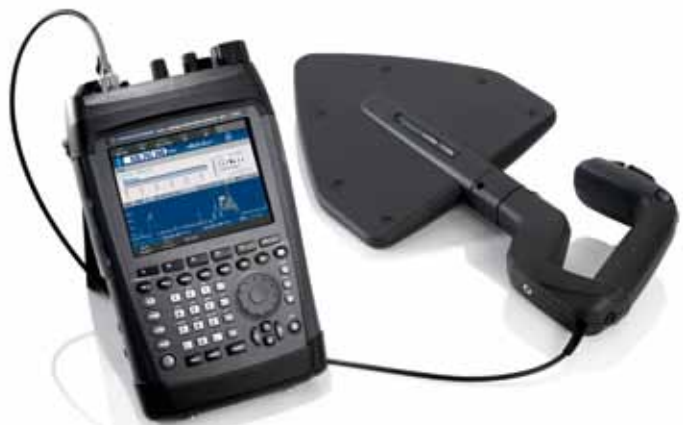
The R&S®PR100 with the R&S®HE300 active directional antenna: The antenna comes with three modules that cover the frequency range from 20 MHz to 7.5 GHz (can be expanded to 9 kHz with optional HF module). The preamplifier is accommodated in the grip piece.
