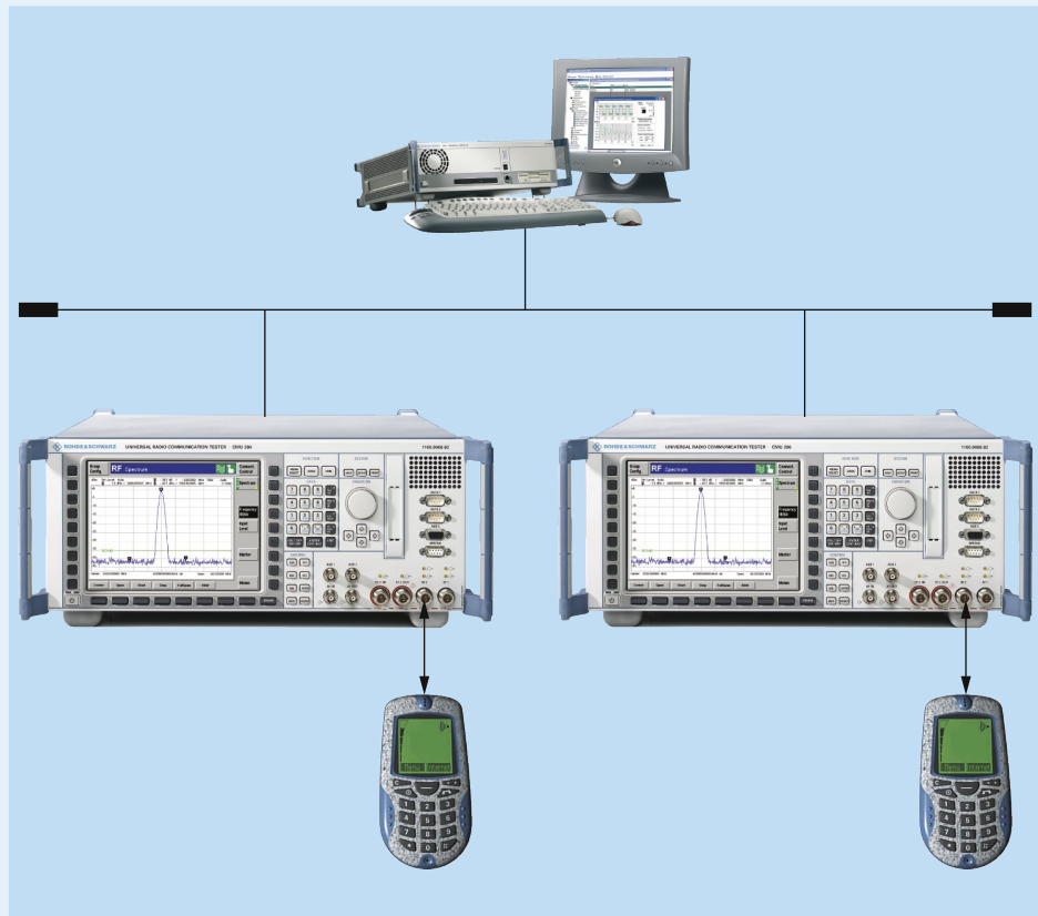
FIG 5 Test setup for data end-to-end tests, for example for testing the exchange of an MMS message between two mobile phones.
