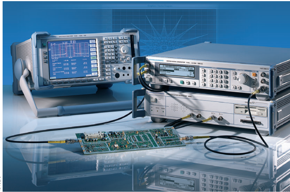
FIG 1 Module test using R&S SMV03, R&S AMIQ and Spectrum Analyzer R&S FSP.
