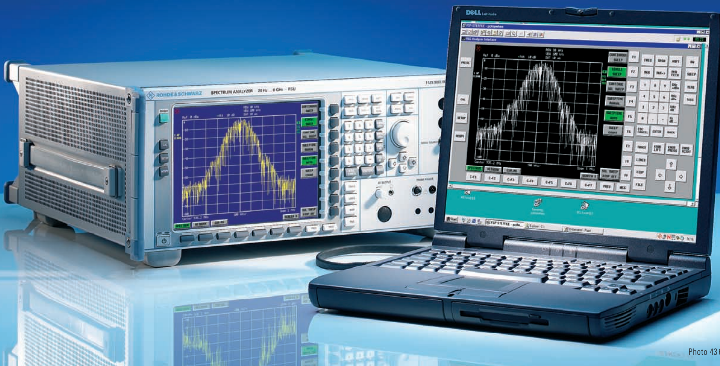
FIG 1 The FSU family consists of two analyzers for the RF range and the lower microwave range: the FSU3 (20 Hz to 3.6 GHz) and the FSU8 (20 Hz to 8 GHz). The PCAnywhere software allows remote control of the analyzers with a mouse.
