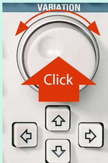
FIG 4 The rotary knob, which can also be pressed, enables you to conveniently navigate within the panels.
