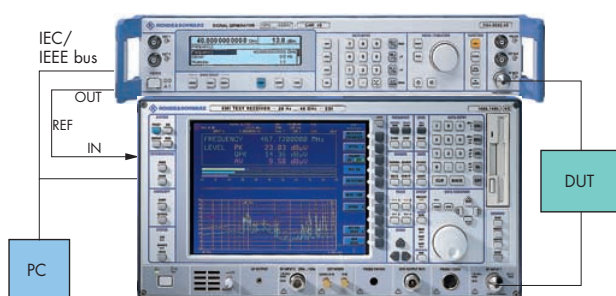
FIG 1 Just a few connections make SMR and ESI ready for user-friendly automatic measurements on microwave components up to 40 GHz
