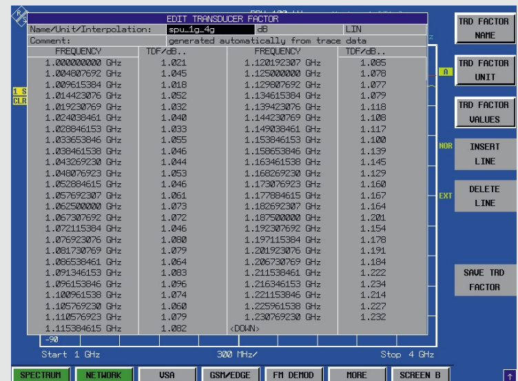
FIG 7 Transducer automatically generated with SAVE AS TRD FACTOR.
