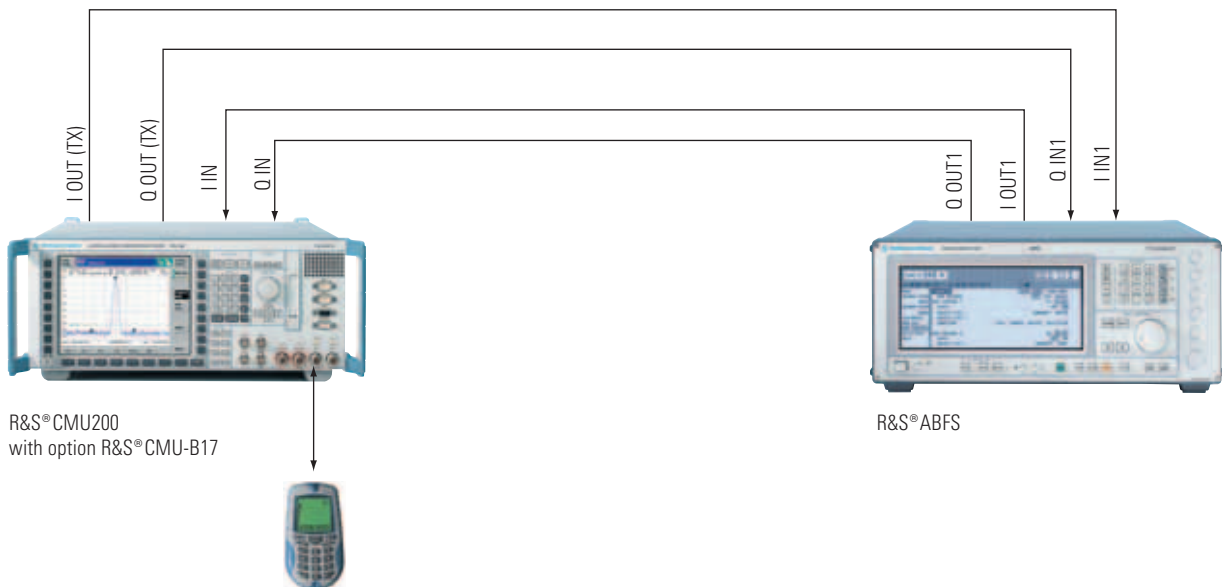
Fig. 2: The R&S® CMU 200 with option R&S® CMU-B17 in combination with the Fading Simulator R&S® ABFS for receiver tests under fading conditions
